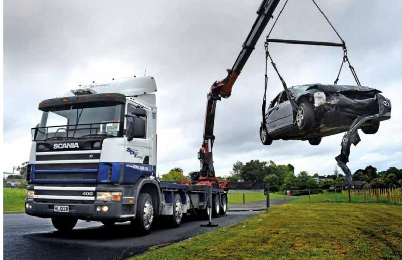
Scania 400 10x4 Hiab unit, capable of lifting up to 12 tonnes close in, recovers a wreck
